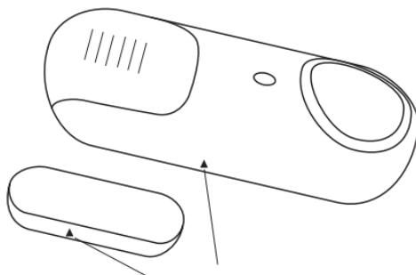
The triangular indicators need to be in line when mounting the magnet and the alarm unit.
